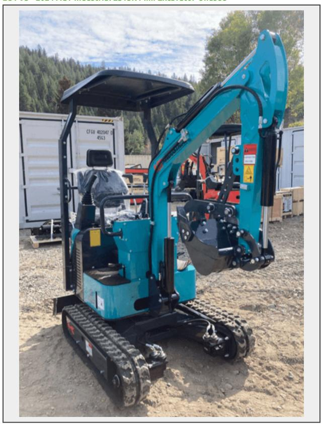
Unused 2024 AGT Industrial LS15R mini excavator, 420cc gas engine, 8.6KW, 15" bucket, 4' tracks, 6" wide tracks, 38.5" base, hydraulic boom and bucket controls, approx. weight 920 kgs.
